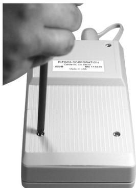
Installation of the battery cover is the reverse of removal. Take care not to overtighten the screws securing the battery cover or damage may result.
