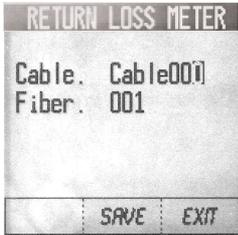
9. To store the test, press the SAVE softkey. The screen will prompt you to identify the Cable & Fiber.
